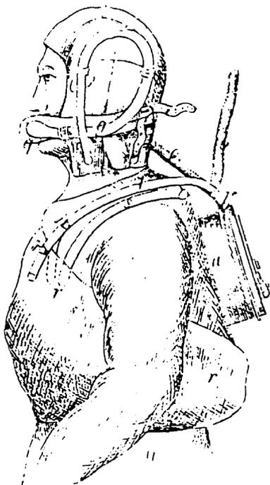
This drawing from Newton's patent specification shows the demand valve on the diver's back and the "stab jacket" on his chest and under his arms with the looped exhaust tube by his head.
